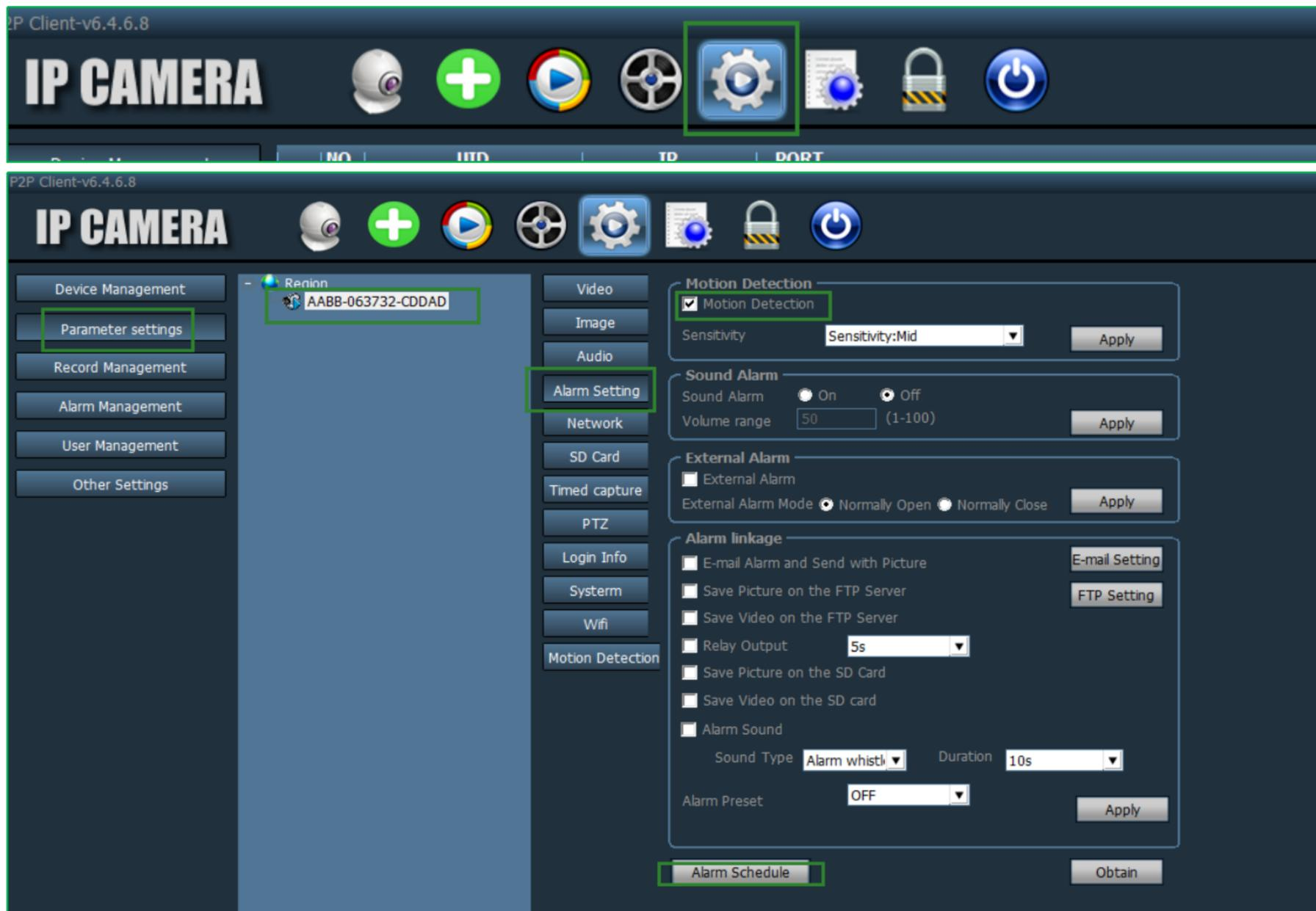
Enable Motion detection in Alarm Setting. You can setup a alarm schedule in Alarm Schedule, click the left mouse to drag a green blocks in the schedule.
