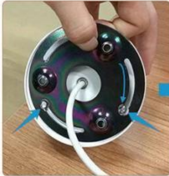
Rotate the base to the position of the arrow and remove it from the tail line
