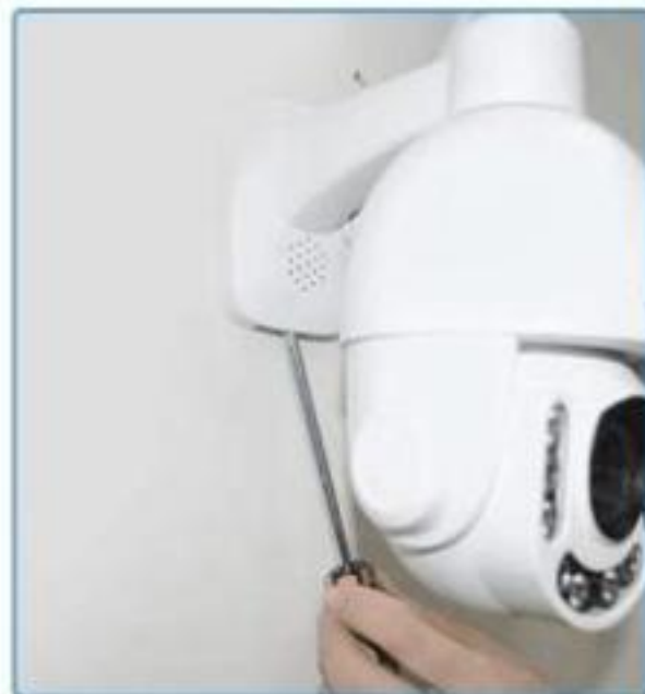
Reattach the base screw
