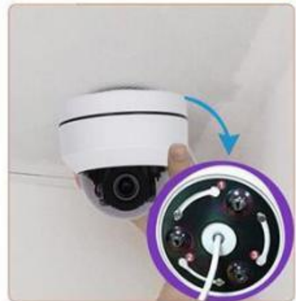
Place the three rounds at the bottom of the PTZ camera at 1, 2, 3, and then turn left to the far left.
