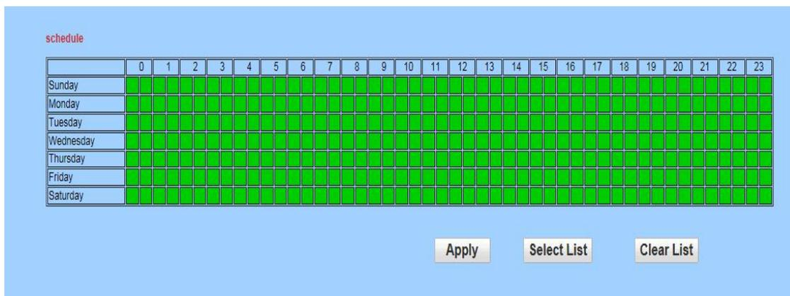
The device will trigger an alarm only when an alarm is detected during a time period when the alarm is set, so you need to carefully choose which time period to set the alarm for.
